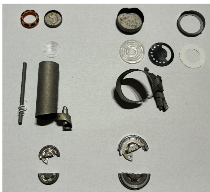
Figure 4. Photographs of teared-down orange (left) and grey (right) cell without jelly roll.
