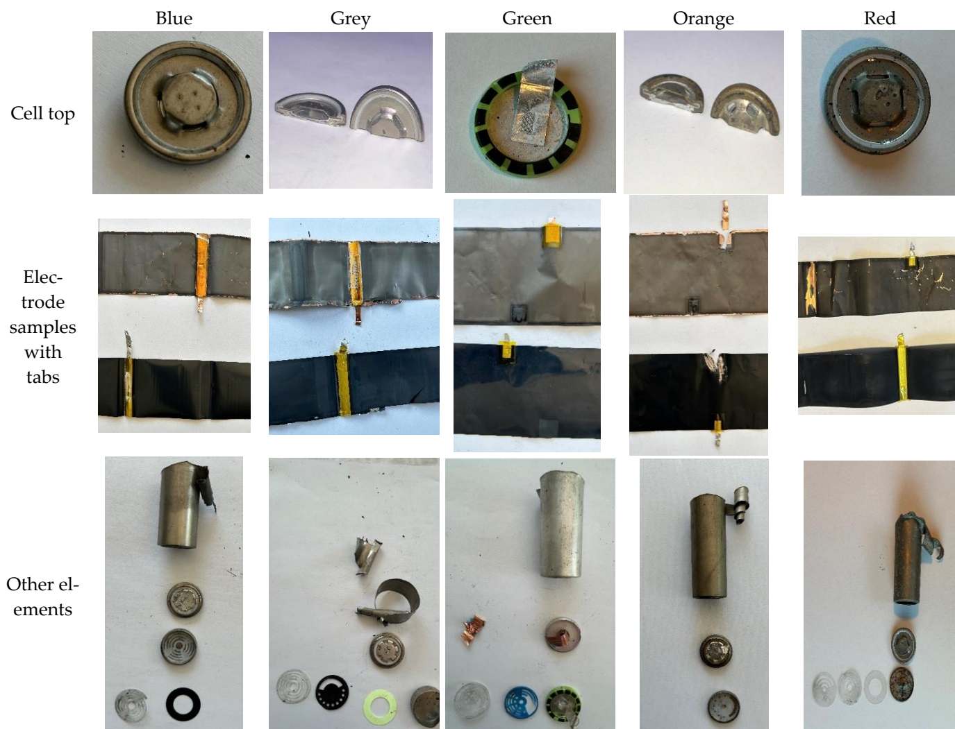
Figure A9. Detail pictures from cell tear-down.
