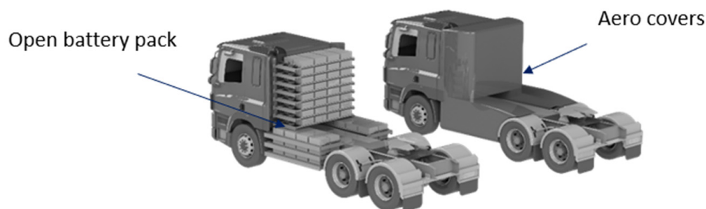
Figure 1. Rendering of the battery pack in the truck with and without aero covers.
