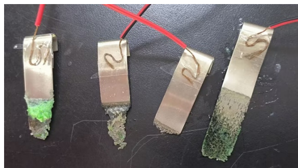
Figure 3. The corroded nickel strip after the discharge in KCl solution. From left to right: 60, 30, 15, and 5 g/200 mL deionized water.
