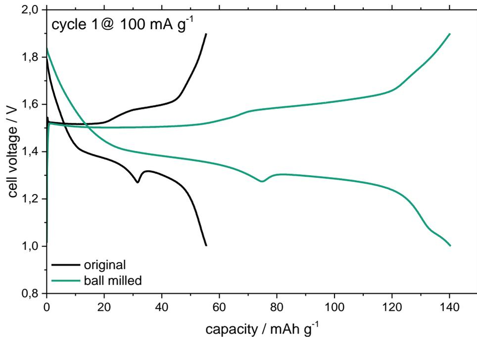
**Figure S3** Cell voltage curves showing the first cycle with an applied current density of  $100 \text{ mA g}^{-1}$  of the cell with original (black line) and ball milled active material (green line). Two voltage plateaus each are visible in charge and discharge step (the voltage plateaus of the discharge steps are divided by a significant voltage drop), which can be dedicated to phase transformations effects.
