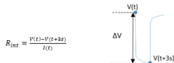
Figure 4. Internal Resistance evaluation during a 3 s resting period.
