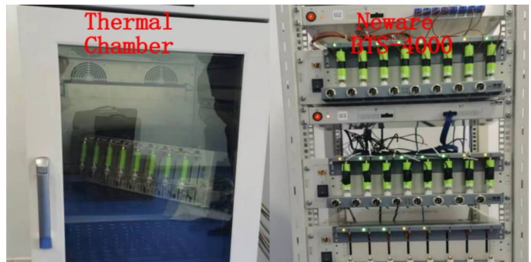
Figure 6. The charge–discharge instrument for lithium-ion battery test.
