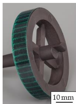
Figure 5. Circular and multipolar sample with a flux foil on the outer diameter to illustrate the magnetic field.
