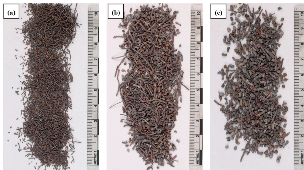
Figure 4. Heavy fractions from CF010-NE after density separation at different particle classifications: (a) 0.50–0.71 mm, (b) 1.00–1.18 mm, and (c) 1.40–2.00 mm.
