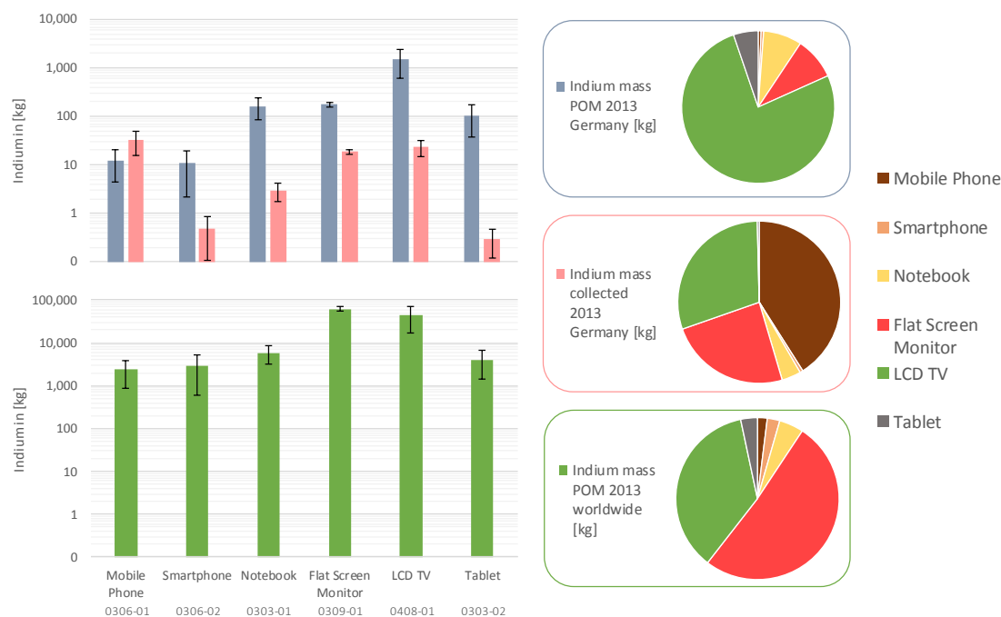
Figure 6. Total indium potential from LCD panels in various put-on-market devices (Germany/worldwide) versus Waste Electric and Electronic Equipment (WEEE) devices collected for recycling purposes in Germany in 2013.
