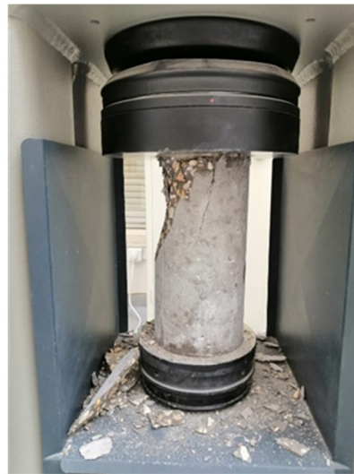
Figure 4. Concrete compression test.
