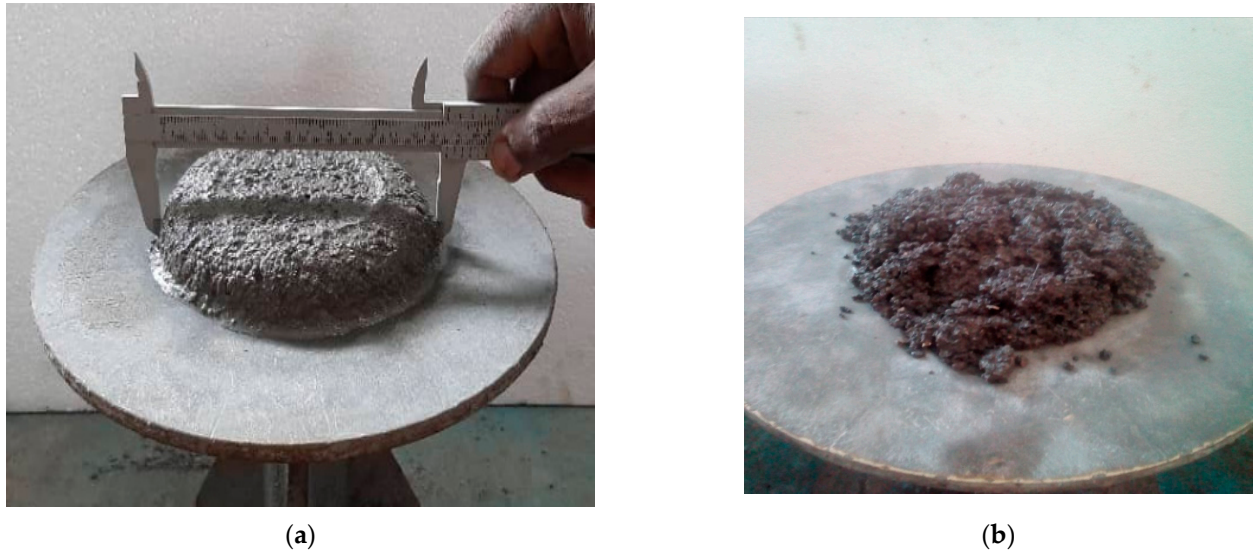
Figure 6. Mortar consistencies: (a) normal flow and (b) scattered flow.
