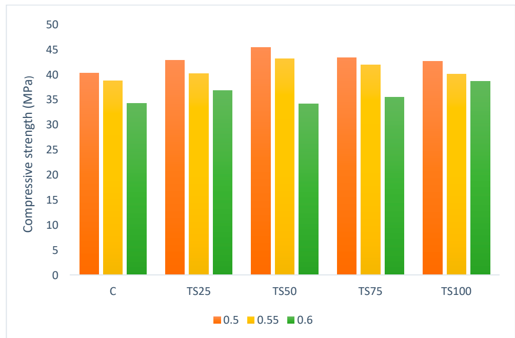
Figure 10. The compressive strength of graded TS at different w/c ratios.
