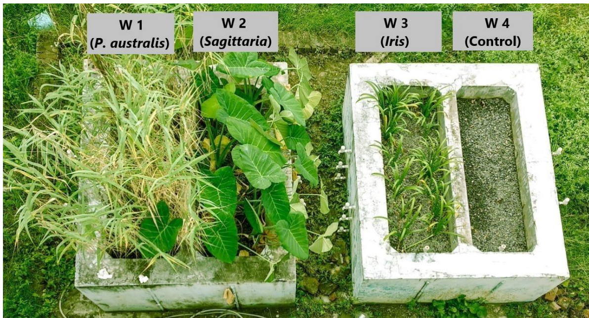
Figure 2. Profile photo of the four beds of HSSF-CWs: W1 ( P. australis ), W2 ( Sagittaria ), W3 ( Iris ), and W4 (Control).
