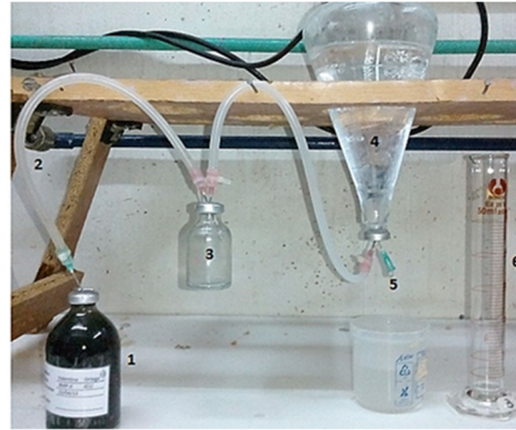
Figure 1. System used for the quantification of methane production by liquid displacement: (1) sample; (2) biogas outlet; (3) trap for liquid; (4) Mariotte bottle with alkaline solution; (5) volume output; (6) probe to measure displaced liquid.
