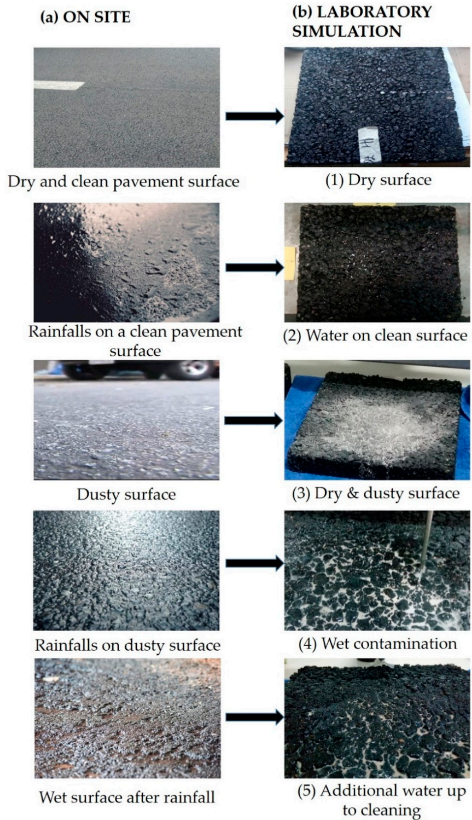
Figure 10. Consideration of various weather conditions: (a) on-site status and (b) laboratory simulations.
