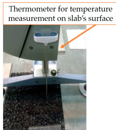
Figure 9. Temperature measurements on the specimen's surface.
