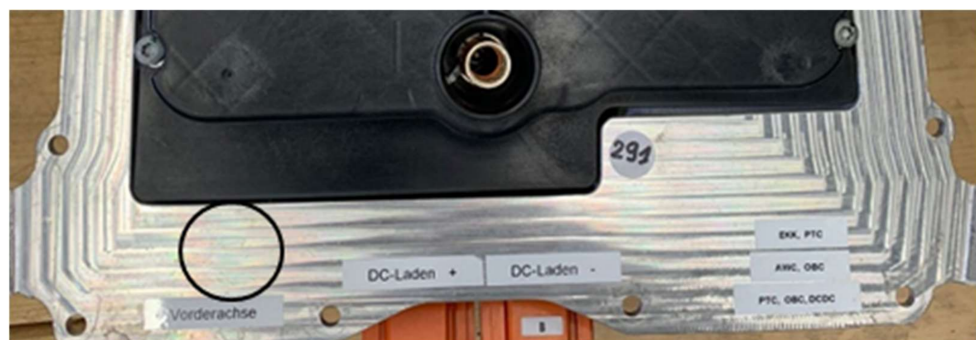
Figure 21. Presentation of the switch box and the black marked measuring points.
