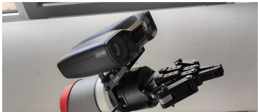
Figure 7. Zivid Two with projector (left) and 2D camera (right) mounted on a robot arm.
