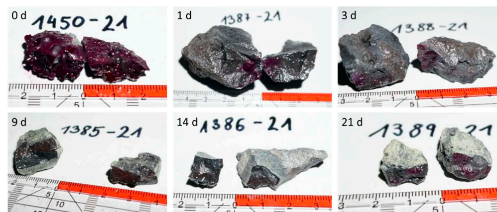
Figure 20. Determination of the carbonation depth using phenolphthalein.
