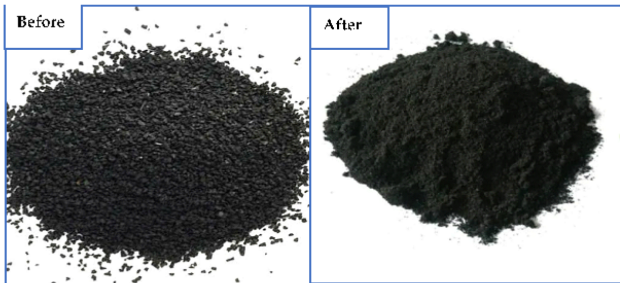
Figure 2. Visual inspection of milled rubber tires (before and after milling).
