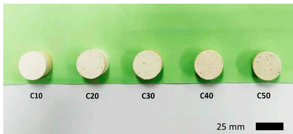
Figure 2. Visual observation of the investigated samples after sintering at 1300 °C for 2 h.
