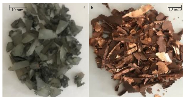
Figure 2. Complete polyurethane material after comminution with separated PUR (a) and Cu (b).
