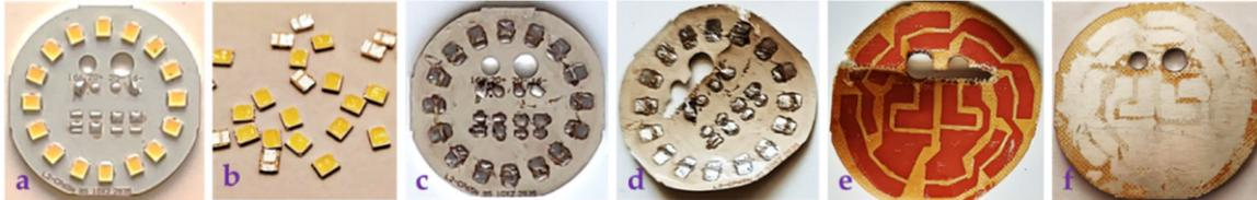
**Figure 7.** (a) “LED module” (E27-C), (b) SMD LEDs, (c) “bare LED module”, (d) top view of the detached PCB, (e) rear view of the detached PCB with the electrical circuit and insulating thin-film coating, and (f) the aluminium substrate of the LED module (authors’ images).
