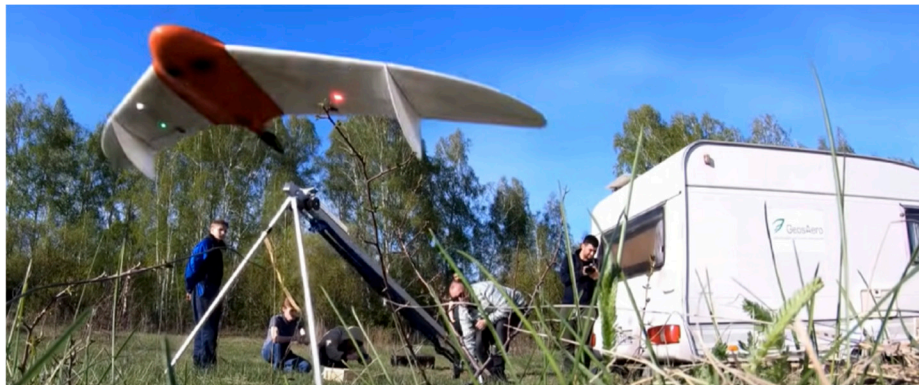
Figure 1. A UAV launching from the launcher.
