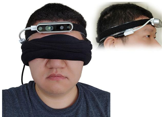
**Figure 9.** Testing configuration of the RGB-D camera worn like a headlamp.
