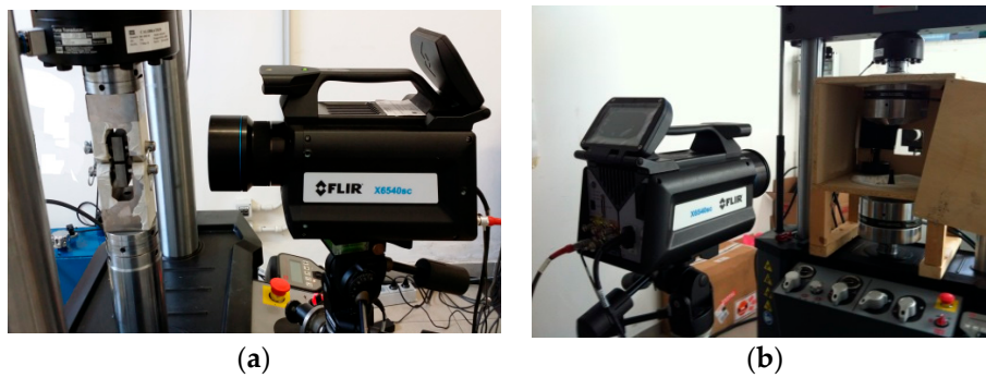
Figure 1. Experimental setup: (a) Fracture Mechanics test; (b) Fatigue test.
