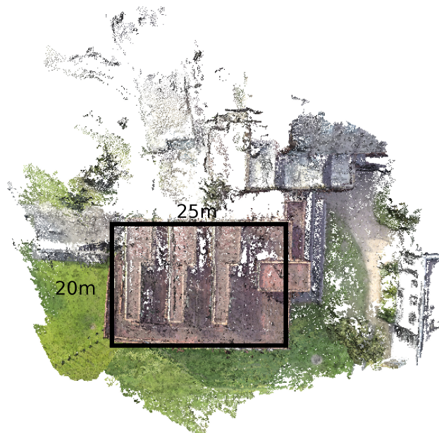
Figure 10. Aerial view of the point cloud in natural RGB color generated by the medium FOV. The black box highlights the area of the target building.
