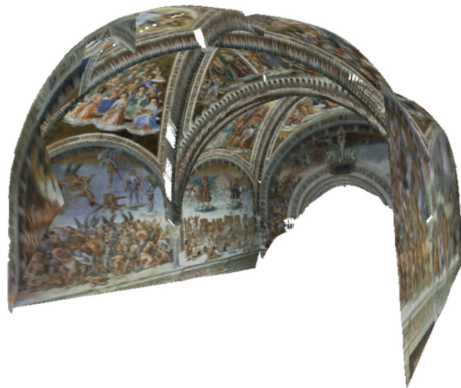
Figure 11. 3D model of the San Brizio Chapel obtained with the RGB-ITR scanner. The colors are uniform without shadows, unlike photographs (Figure 9). (Elaboration carried out by ENEA team with the custom software itrAnalyzer).
