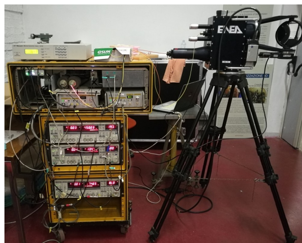
Figure 2. RGB-ITR (Red Green Blue-Imaging Topological Radar) scanner prototype in a laboratory environment, set up with the optical head on a tripod and the electronic components in the tower configuration.
