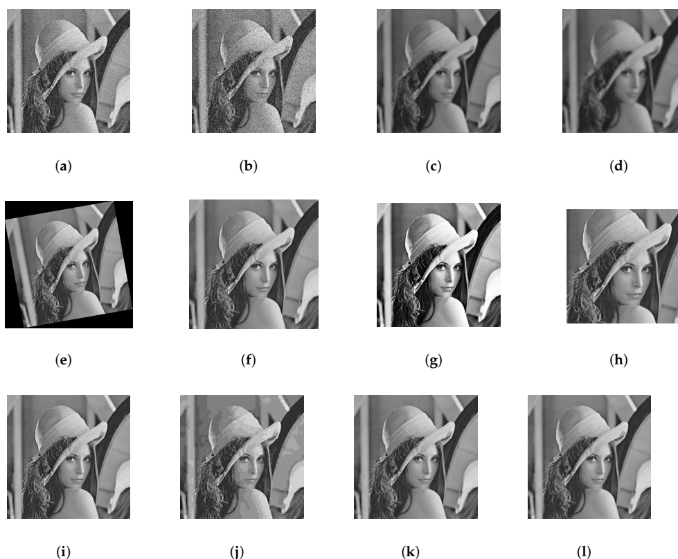
Figure 12. Sample of attacked watermarked images: (a) Gaussian noise addition with zero mean and standard deviation (0.01), (b) Salt and pepper noise with noise density 0.01, (c) Low-pass Gaussian filtering ( \sigma = 0.5, 7 \times 7 ), (d) Low-pass Gaussian filtering ( \sigma = 0.6, 7 \times 7 ), (e) Rotation ( 10^\circ ), (f) Scaling (1.2), (g) Histogram equalization, (h) Cropping(25%), (i) JPEG compression with quality factor 60, (j) JPEG compression with quality factor 5, (k) Gaussian smoothing ( \sigma = 0.7, 7 \times 7 ), (l) Gaussian smoothing ( \sigma = 0.9, 7 \times 7 ).
