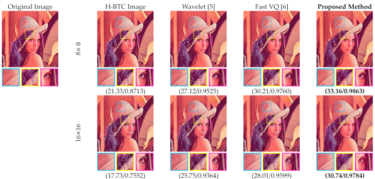
Figure 15. Visual comparisons between the proposed method and former schemes on reconstructing the DDBTC decoded image over the Lena image.
