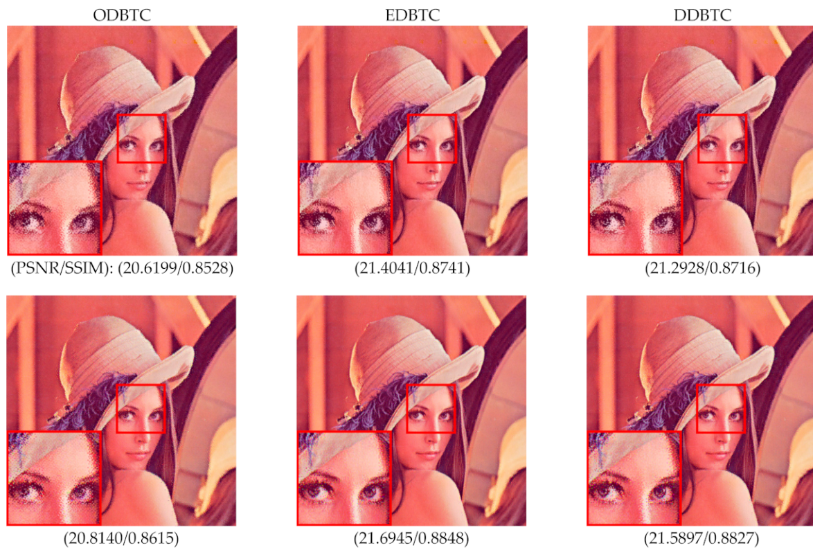
Figure 2. Visual comparisons of using single and three bitmap images on (first to last column) ordered dither block truncation coding (ODBTC), error diffusion block truncation coding (EDBTC), and dot diffused block truncation coding (DDBTC). The first and second rows are using single and three bitmap images, respectively.
