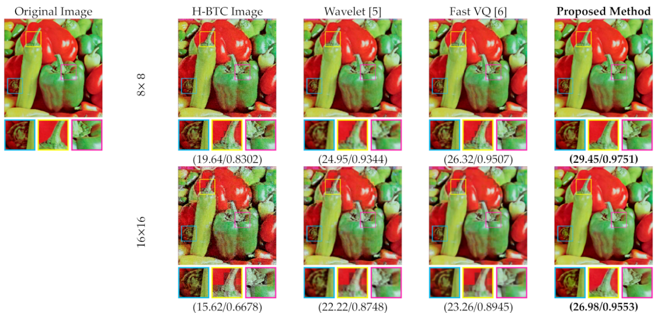
Figure 16. Visual comparisons between the proposed method and former schemes on reconstructing the DDBTC decoded image over the Peppers image.
