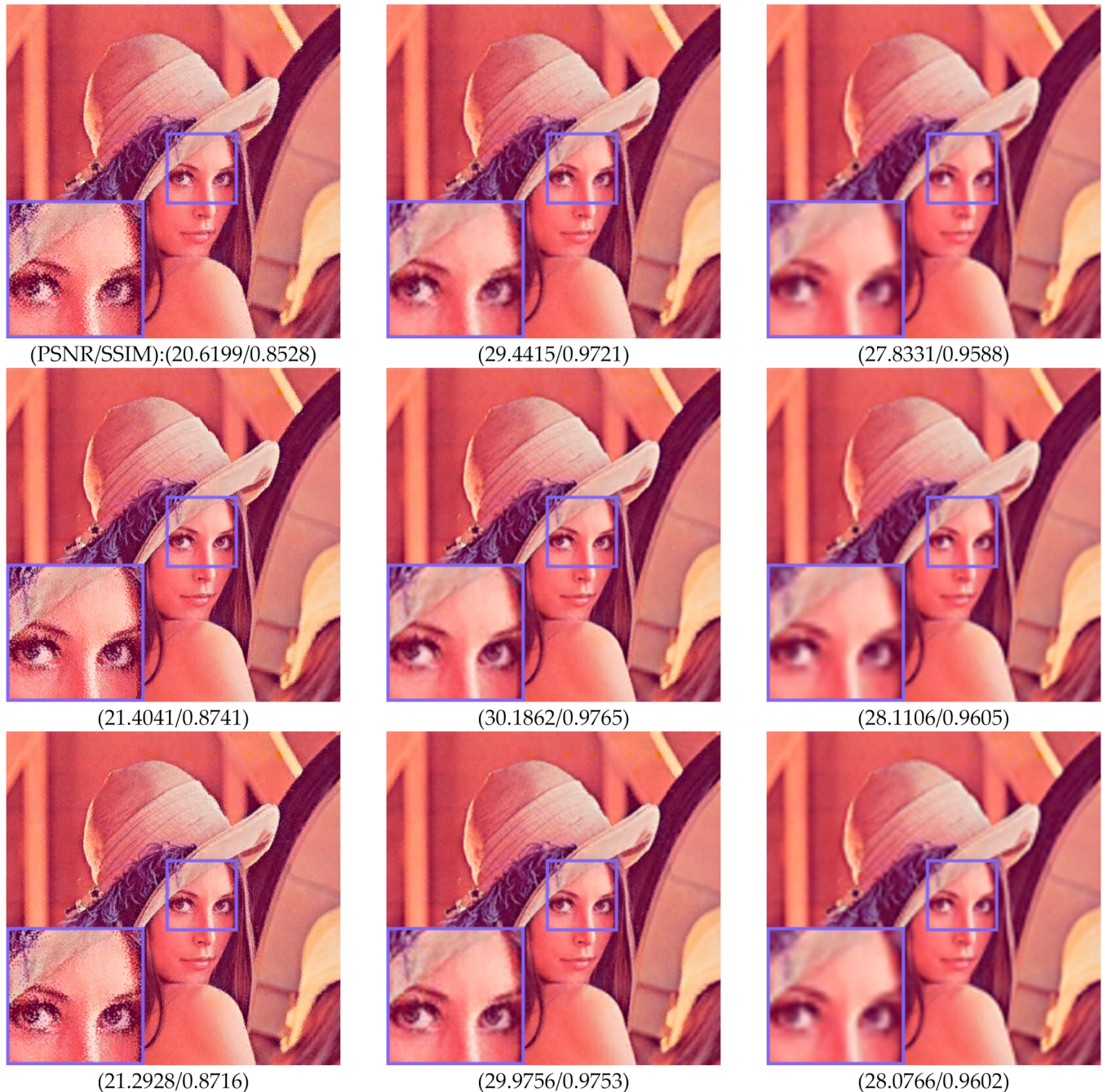
Figure 5. Effects of performing downsampling and upsampling operations on (first to last rows) ODBTC, EDBTC, and DDBTC. The first column is the original decoded image. The second column are reconstructed images after applying downsampling with factor 0.5 and upsampling to the original size, while the third column are images after downsampling operator over factor 0.25 and upsampling to the original size.
