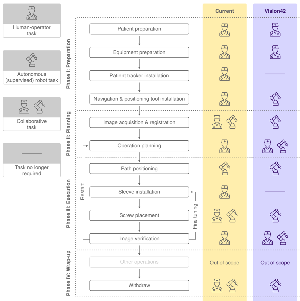
Figure 3. Workflow phases, subordinate steps and human-robot collaboration levels of a current PSP procedure [6] (yellow) and a futuristic PSP procedure (violet). The icons used are explained in the legend on the left.
