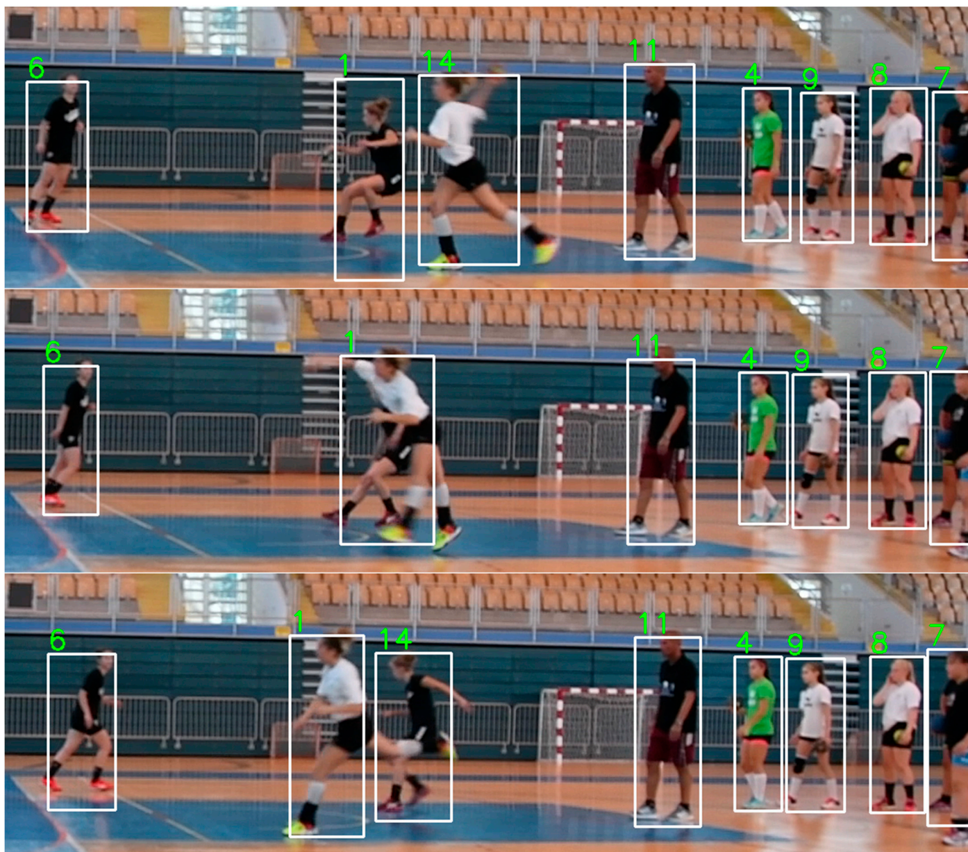
Figure S9. Example of scenario where Tracktor++ tracker performs poorly. Tracktor++ performs well when tracking the players while running across the field but struggles when the players occlude each other. In this example, Tracktor++ switched the ids of players with ids 1 and 14 after one player passed in front of the other. Given that Tracktor++ combines motion-based and feature-based tracking, it is unexpected that this kind of error occurs when players have different appearances and motions. Tracktor++ is less sensitive to poor consistency of bounding box detection than other methods because it uses feature-based tracking that helps to retain object id even when the bounding box changes size and shape.
