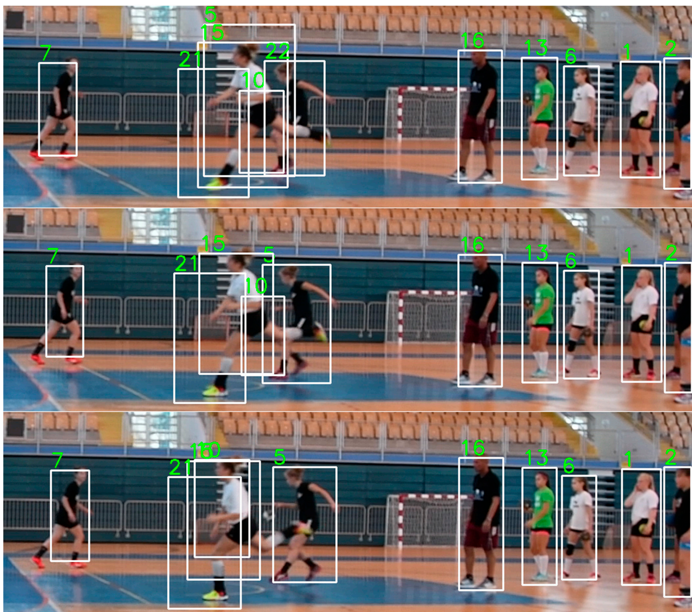
Figure S8. Example of scenario where DeepSORT tracker performs poorly. DeepSORT continues to track players that do not exist, producing a lot of False Positives, but even in that chaos, it continues to track the player with the id of 15 while it passes in front of the other player. However, the player with the id of 22 in the first row changes the id to 5 in the following two rows, meaning that DeepSORT did not manage to capture a robust enough feature representation that recognizes the object even when partially occluded. DeepSORT is less sensitive to poor consistency of bounding box detection than other methods because it uses feature-based tracking that helps to retain object id even when the bounding box changes size and shape.
