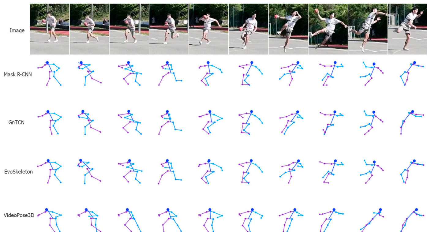
Figure S1. 3D pose estimation by models GnTCN, EvoSkeleton and VideoPose3D using 2D keypoints produced by Mask R-CNN . The right side of the player is colored purple while the left side of the person is colored blue .
