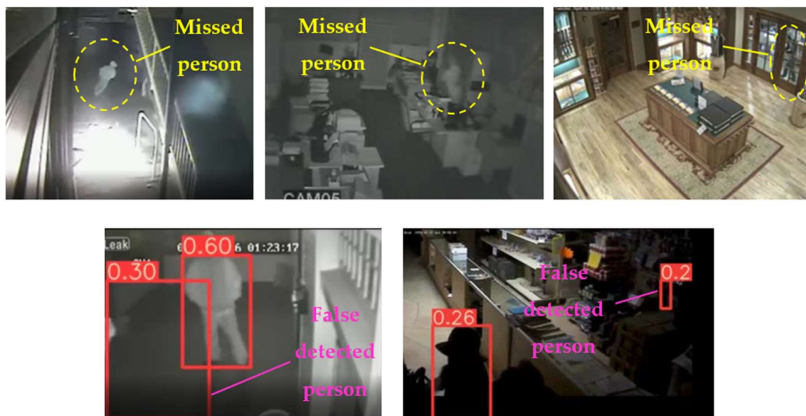
Figure 12. Observed FN entries (yellow ellipse with dashed line) and FP entries (magenta indications) during the person detection process applying the pre-trained YOLOv5s.
