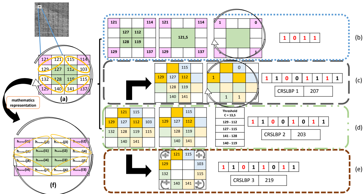
Figure 1. (a) The 4 \times 4 sub-block of the image. (b) The corner processing. The process of the first (c), second (d), and third (e) generated CRSLBP code. (f) mathematical representation of the block.
