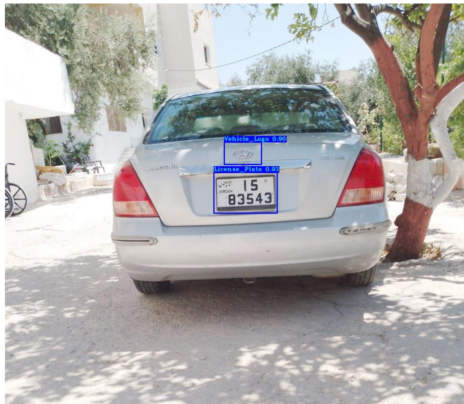
Figure 2. Outputs of the re-trained YOLOv3 model for the Jordanian LPD and VLD tasks. Note that the word “الأردن” is JORDAN.
