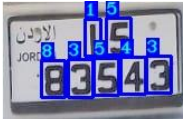
(a) Outputs of the re-trained YOLOv3 model for the Jordanian LPR (CR).
