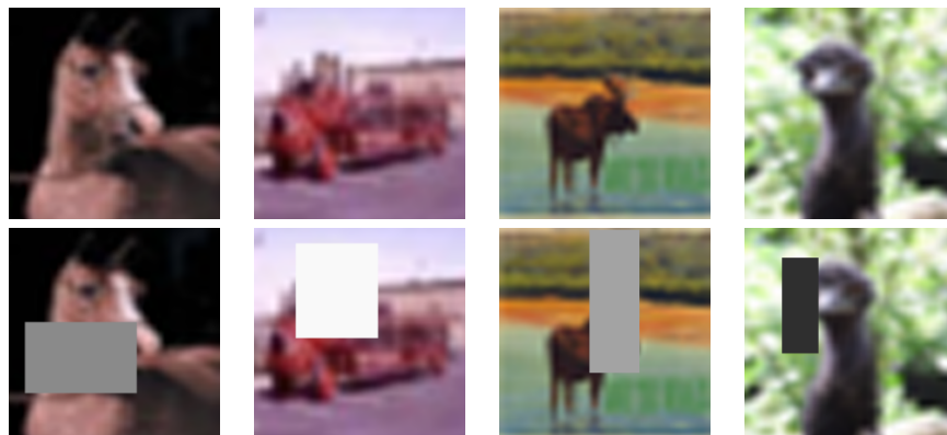
Figure 11. Data augmentation by the random erasing technique. The first and second rows represent the given images (from CIFAR-10) and the images after random erasing, respectively.
