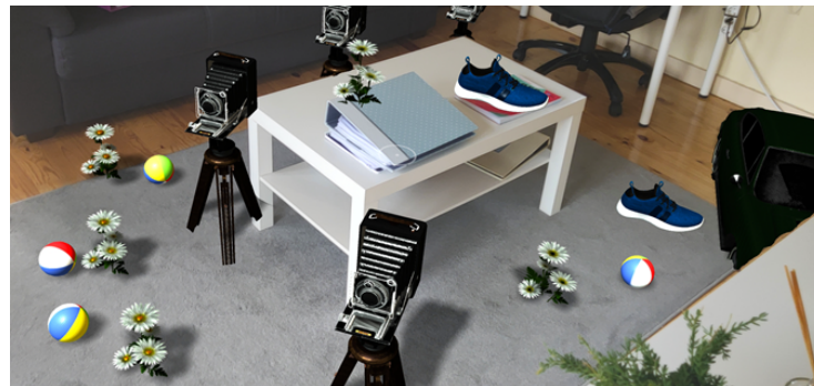
Figure 2. Environment-aware augmented reality rendering with geometry occlusion, shadow casting, lighting matching, and physics interaction between virtual and real world objects.
