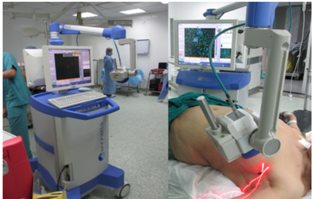
Figure 2. The Sentinella 102 intraoperative gamma camera. This arm-based gamma–optical device can project a laser cross-mark, placed at the centre of the gamma FOV, onto the imaging field. Reproduced from Ibraheem et al. [12].
