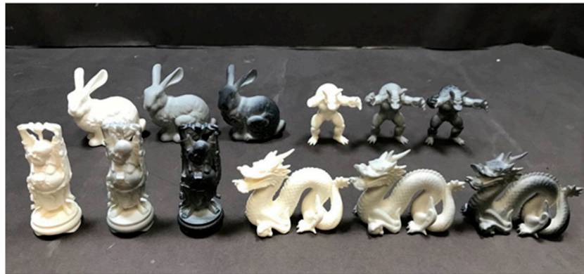
Figure 7. Fabricated samples. For each geometry, from left to right, the order is without texture, with texture 1, and with texture 2.
