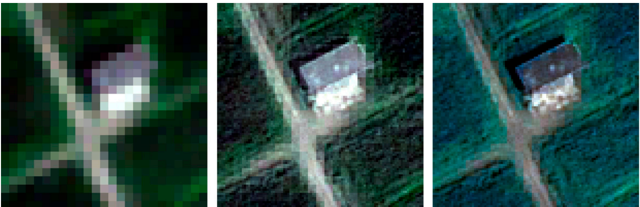
Figure 10. A detail of frame 2: on the left, the RGB composition of the MS images; in the middle, the RGB composition of IHS pan-sharpening; on the right, the RGB composition of BTF pan-sharpening.
