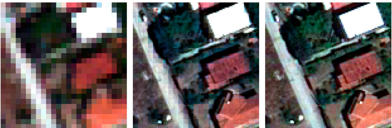
Figure 11. A detail of frame 3: on the left, the RGB composition of the MS images; in the middle, the RGB composition of SFIM pan-sharpening; on the right, the RGB composition of IHSF pan-sharpening.
