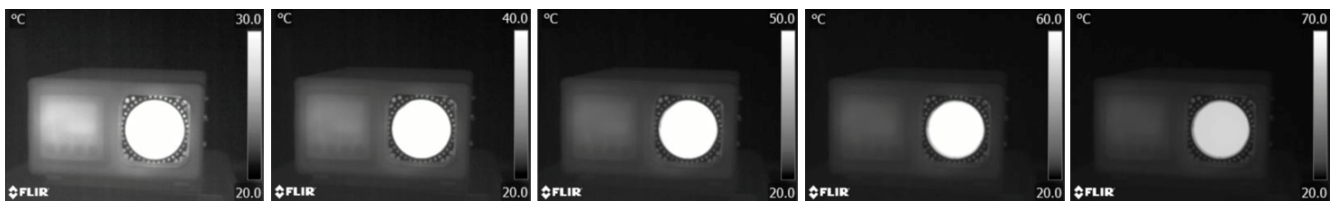
Figure 10. Display of increasing the temperature range by ten degrees °C from the lowest temperature to the maximum registered value.
