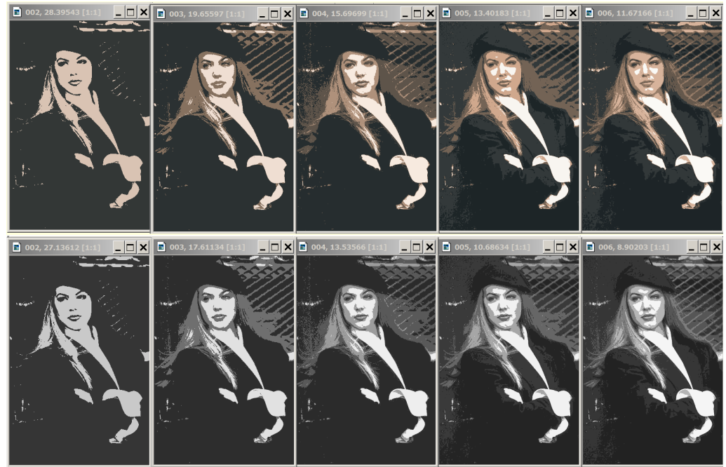
Figure 8. Comparison of optimal approximations for color and grayscale image representations. In the upper row, the optimal color image approximations in g = 2, 3, 4, 5, and 6 colors are presented from left to right, and, below them, similar approximations of the grayscale image are shown. Image approximations at the top are labeled with g cluster numbers and standard deviation values \sigma .
