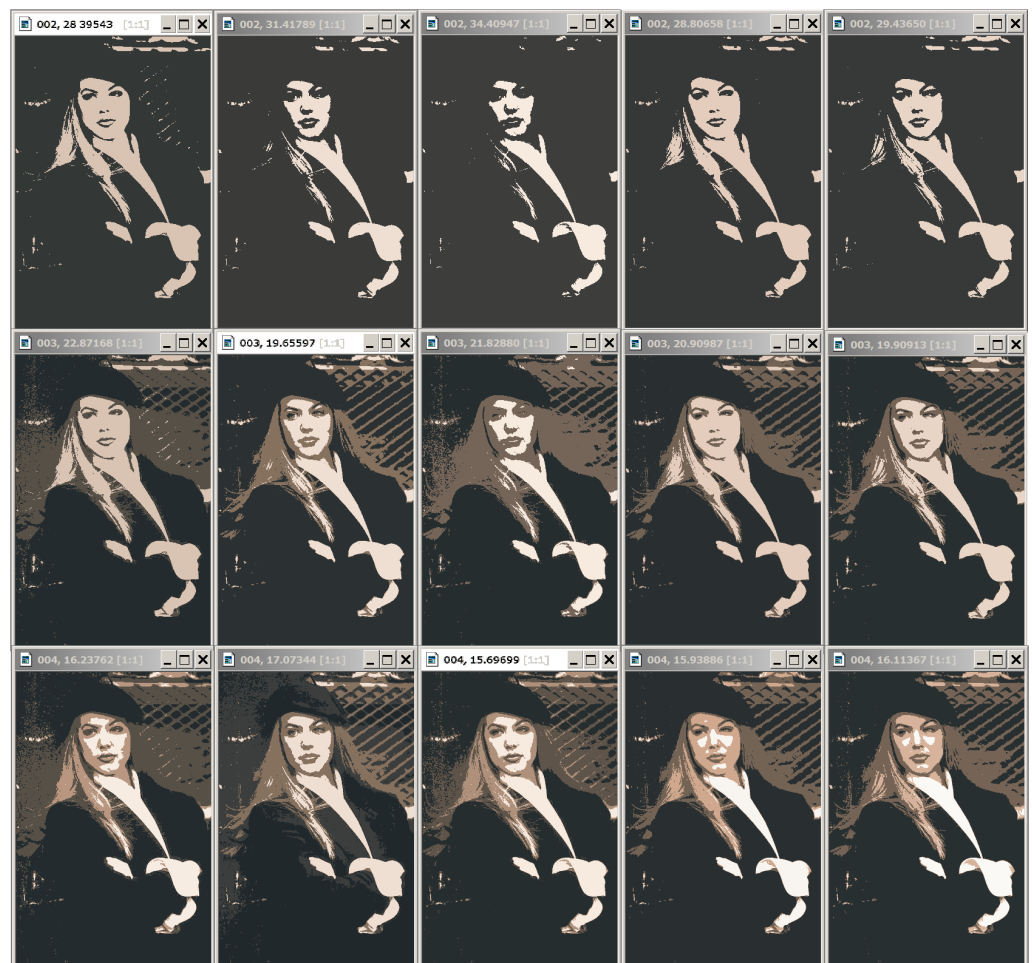
Figure 11. Dynamic Table of approximations for “Girl” color image (dimensions 321 \times 481 pixels). The first row and first column of the table were cropped. The columns of Dynamic Table, containing the optimal image approximations in 2–6 colors, are shown. Each column contains a binary hierarchical sequence of image approximations with incrementally added colors: g = 2, 3 , and 4. On the main diagonal of the Dynamic Table are the optimal image approximations in g_0 = 2, 3 , and 4 colors. Image approximations at the top are labeled with g color numbers and corresponding standard deviation values \sigma .
