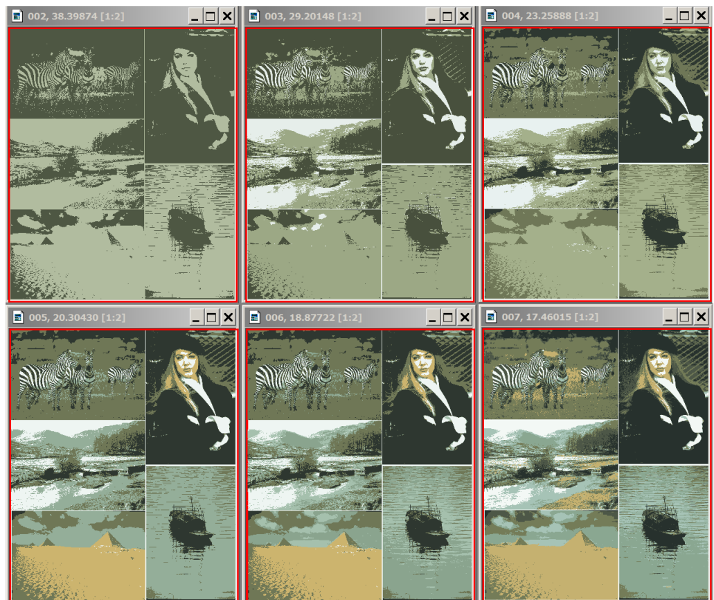
Figure 10. Optimal approximations of “5images” picture in two to seven colors arranged in two rows in lexicographic order. Image approximations at the top are labeled with g color numbers and standard deviation values \sigma .
