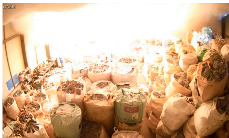
Figure 1. Dust explosion in a magnesium recycling plant (2016) (Photo by Miryang fire department).
