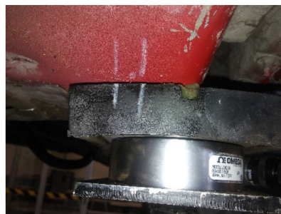
Figure 6. Reference lines on the support pad and the chassis before the test, along the x axis.
