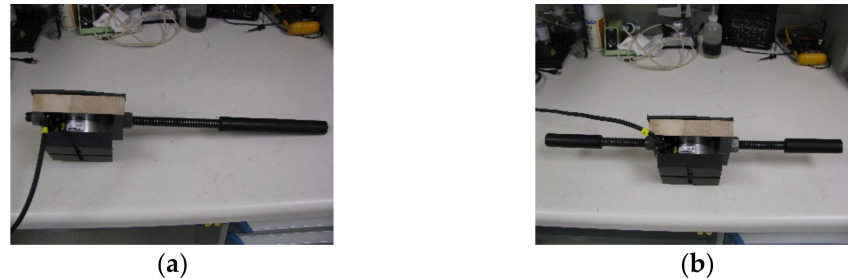
Figure 5. (a) Load cell assembly for lateral force applied to the rear wheel. (b) Load cell assembly for vertical force applied to the trunk.
