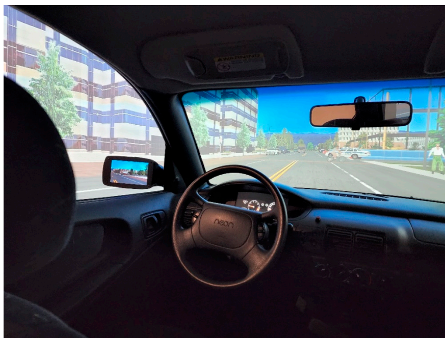
Figure 1. A high-fidelity driving simulator operating in an autonomous mode.
