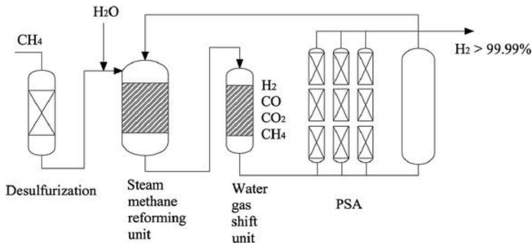
Figure 5. The block diagram of hydrogen generation by steam methane gas reforming [39].
