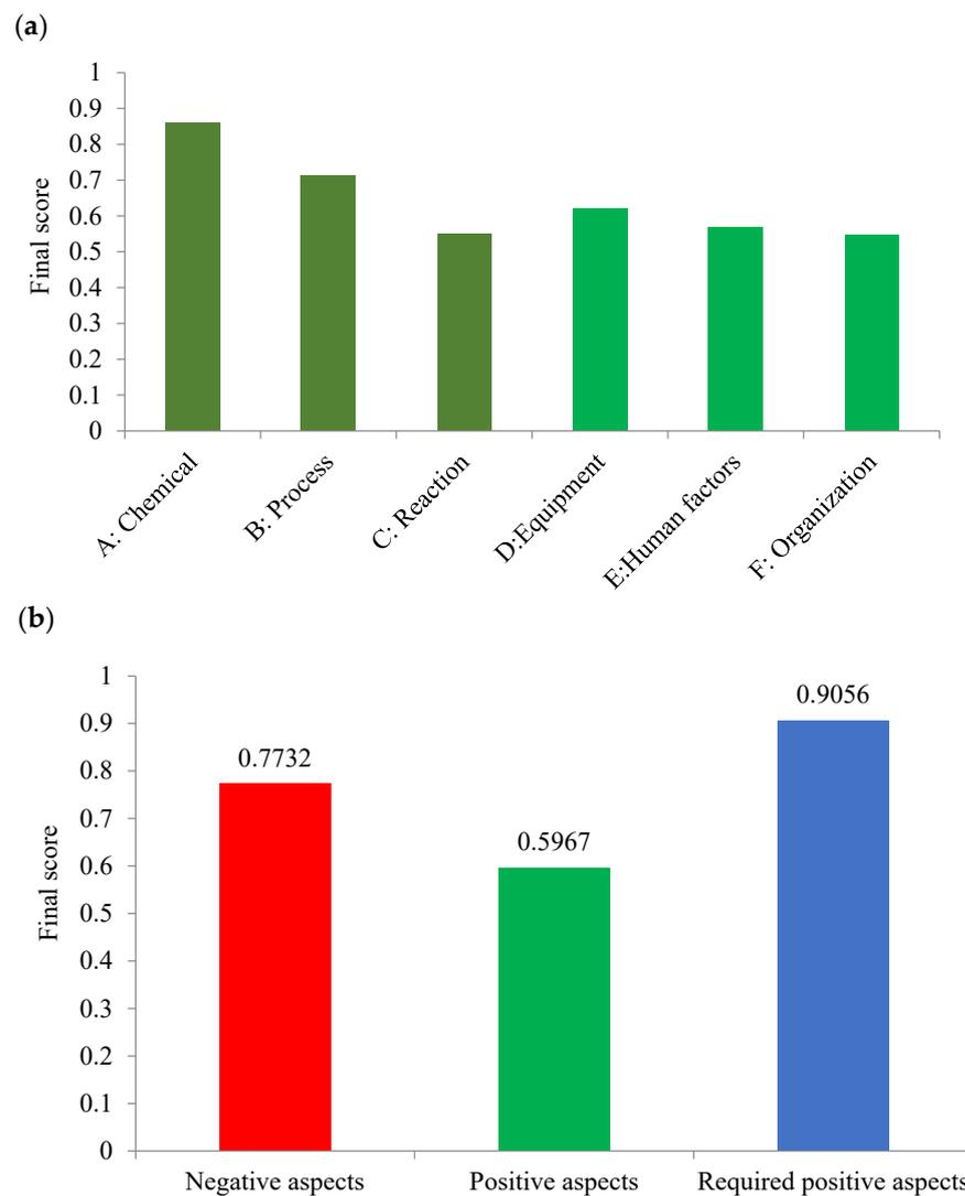
**Figure 6.** The estimated scores of (a) contributing factors and (b) dimensions of ISA in the hydrogen production unit.
