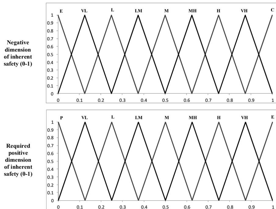
**Figure 4.** The membership function of fuzzy sets of the required positive side of the inherent safety situation.
