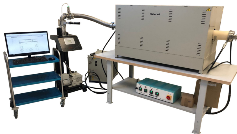
Figure 3. Tubular furnace used for the thermochemical treatment with heating and cooling rate control.
