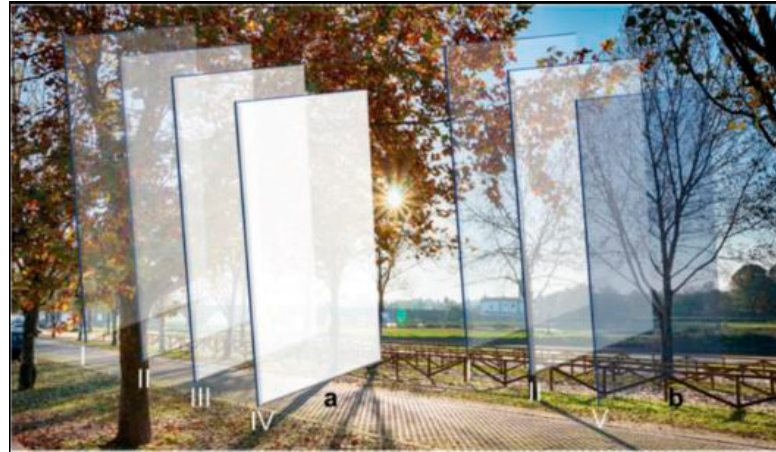
Figure 5. Schematic representation of an integrated system featuring an electrochromic device, which adjusts its transparency to become translucent (a), and a thermochromic device, which changes colour and transparency based on the solar radiation it receives (b) [31].
