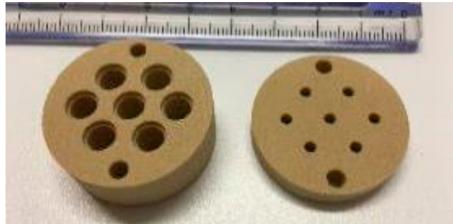
Figure 5. Lens side of the seven-lens sensor head (left), and POF side of sensor head (right).
