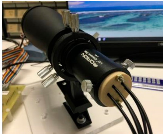
Figure 4. Sensor head installed in Orion 70 mm Multi-Use Finder Scope with fiber optic guides exiting the rear.
