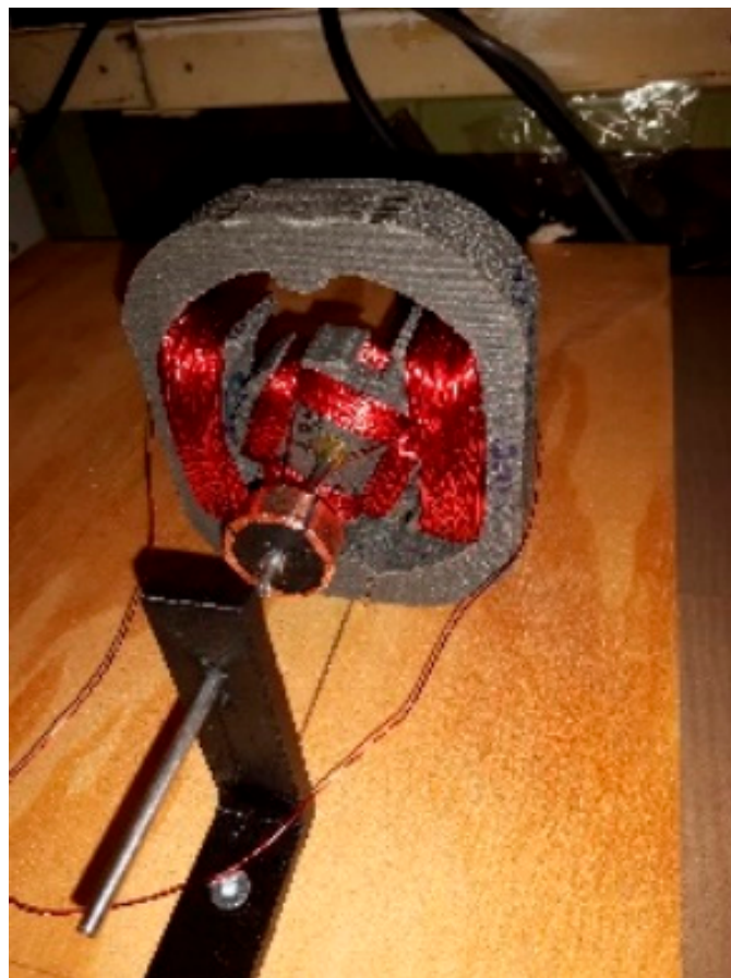
Figure 4. FDM-printed rotor and stator of Fe particles embedded in PLA matrix.
