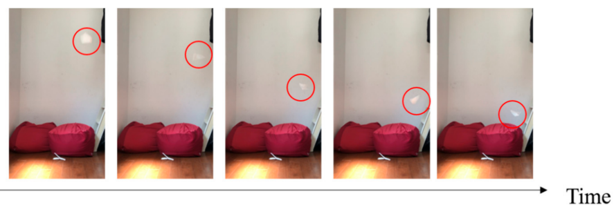
Figure 2. Falling test of the model of the maple tree.
