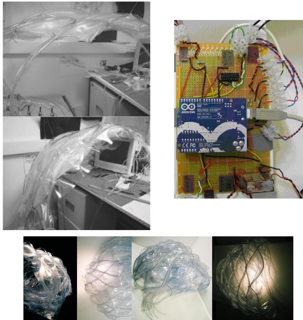
Figure 4. (top left) Dynamic membrane models at 1:5. (top right) Connections, Arduino for the performance of the 1:5 scale model; Circuit composed by: solenoid valve (18 V), motor (3 V), and several LEDs and several resistances. (Below) Static models scale 1:20.
