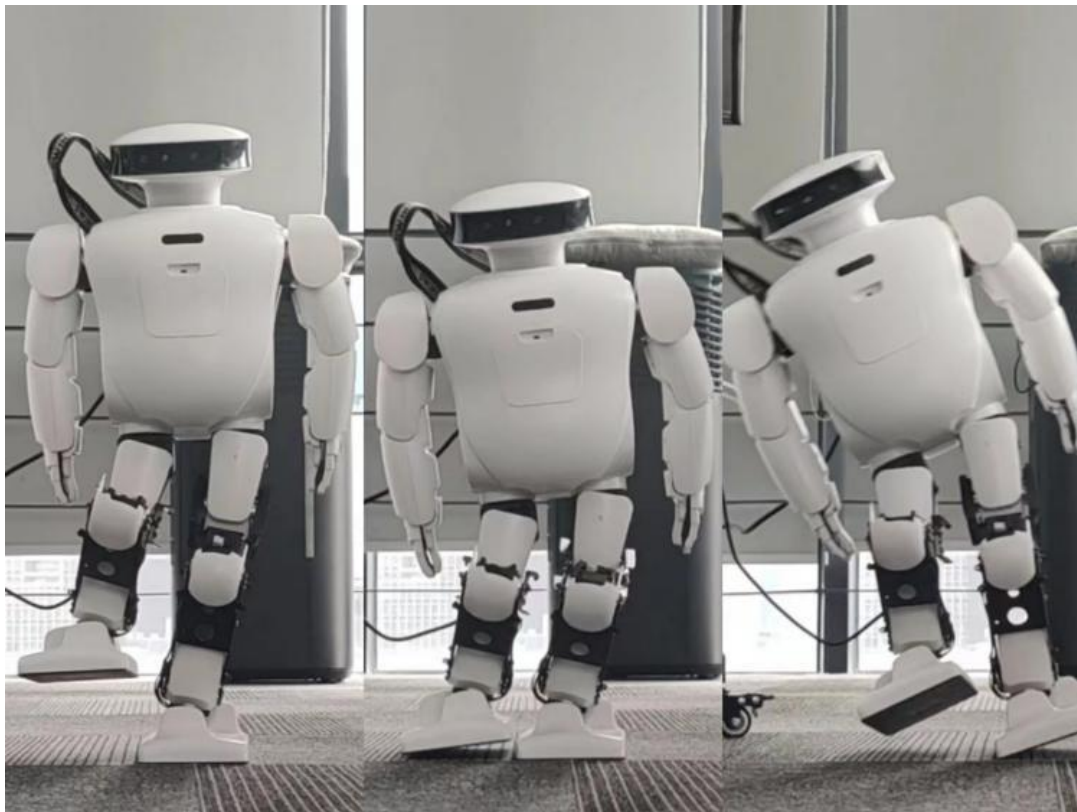
Figure 22. The robot fell down while performing a deeper squat.
